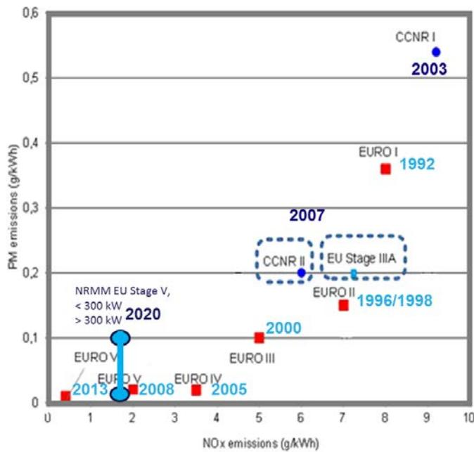
Figure 2: Emission limit comparison between trucks and engines applied in IWT.
