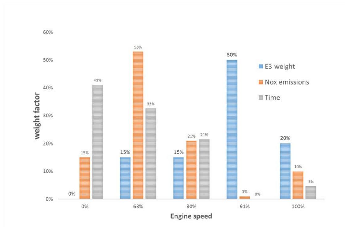
Figure 8: Example of E3 weight factors, compared to sailing time and NOx emissions for the different load points of the E3 cycle
