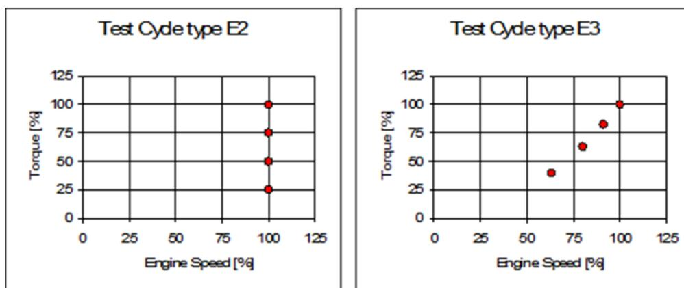
Figure 4. Standard ISO test cycles for vessels
