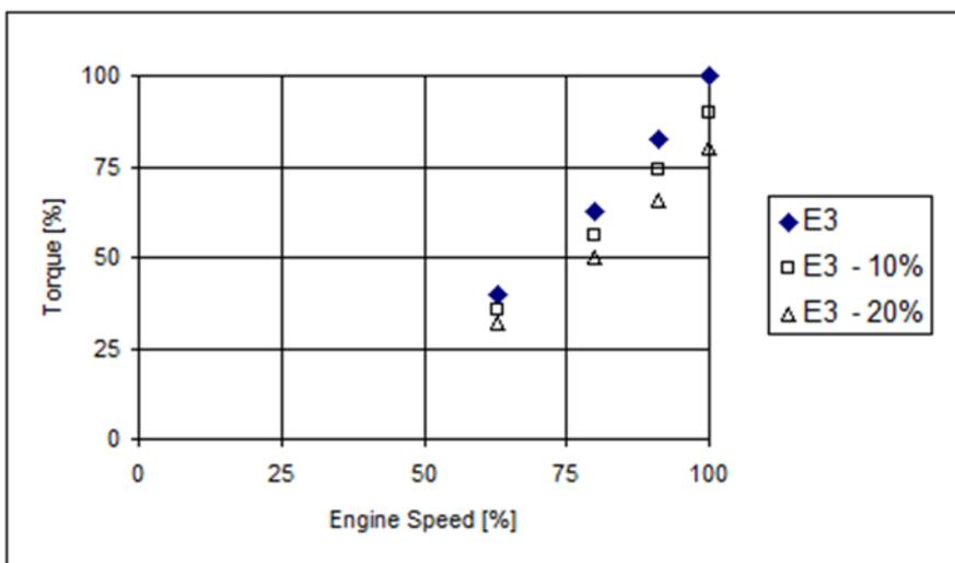
Figure 6. Possible matching deviation of E3 cycle points with an on board measurement
