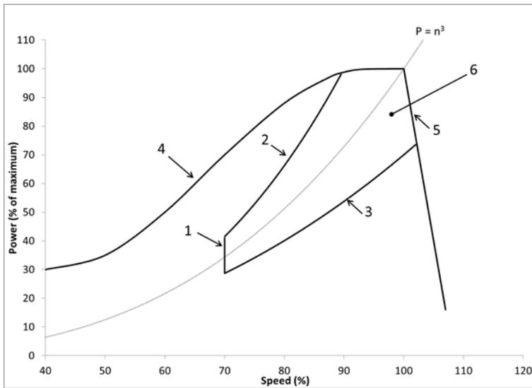
Figure 5. Engine control area of vessel with direct propulsion.
