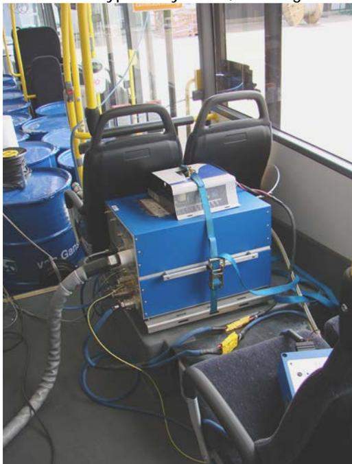
Figure 2. Portable Emissions Measurement System (PEMS) mounted in a bus
